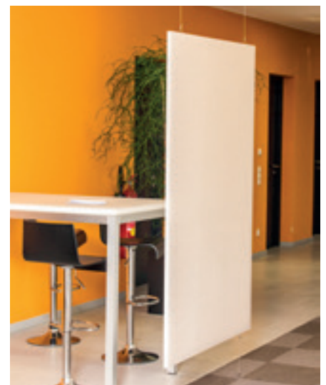
Suspended partition: 1,800 x 1,200 x 25 mm, panels including edge sealing "satin", ceiling and floor suspension (1.5 mm stainless steel cable).
